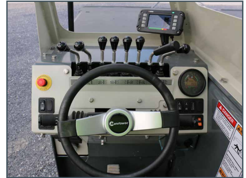
Operator's cab with Rayco-Wylie RCL and mechanical lever proportional controls.
