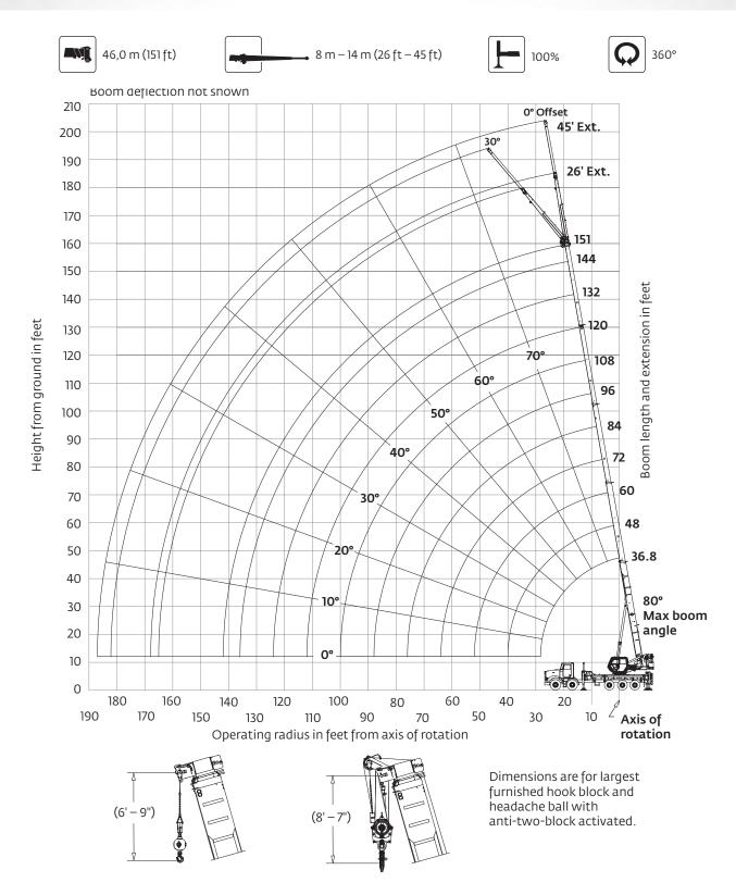
\*This drawing shows the physical reach of the machine. Always refer to load chart to see which portions of this diagram are valid for the specific machine configuration and where the loads are structurally or stability limited.
