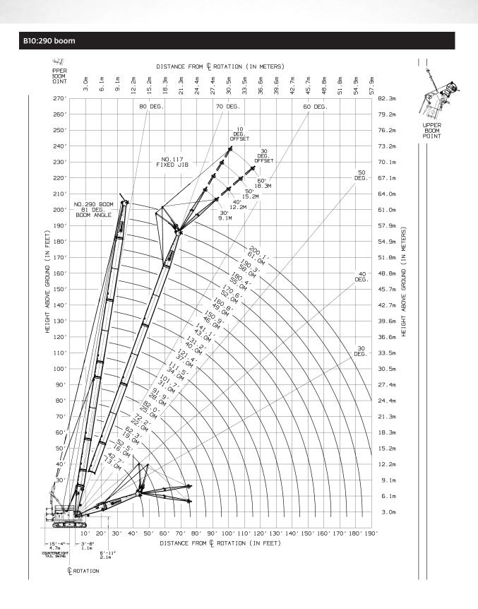
THIS CHART IS ONLY A GUIDE AND SHOULD NOT BE USED TO OPERATE THE CRANE.
