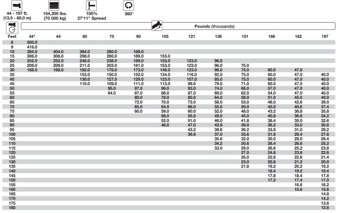
†500,000 lbs is a Comparative Rating. Lifting capacities greater than 350,000 lbs. require additional equipment. Note: Above chart also available with reduced outriggers.
