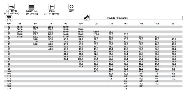
Lifting capacities greater than 350,000 lbs. require additional equipment. Note: Above chart also available with reduced outriggers.
