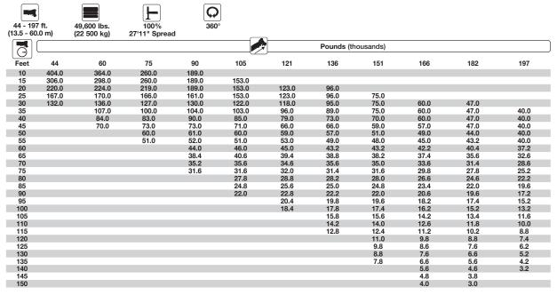
Lifting capacities greater than 350,000 lbs. require additional equipment. Note: Above chart also available with reduced outriggers.
